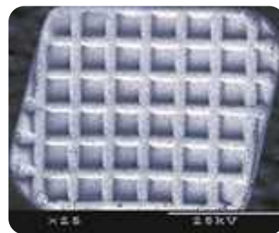
SEM of Di-MIM Micro-Etched Grip-LOK Base
